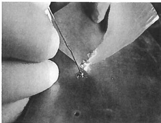
FIGURE 3.—Packing weighed MT into a Silastic tube; the spilled MT was later collected and added to the tube.
