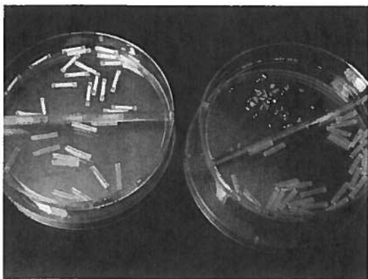
FIGURE 1.—The petri dish on the right contains 12-mm segments of Silastic tubing in one chamber and 1-mm lengths of Silastic rod in the other; the lower chamber of the petri dish on the left contains tube segments with one end plugged and ready for packing, while the upper chamber has finished implants containing 5 mg of 17\alpha -methyltestosterone (MT).
